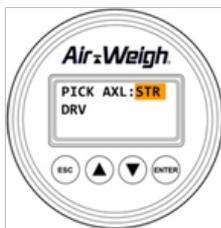
8. Use the up and down arrows to select the weight adjustment you want to make. Press ENTER once the weight is reached. The screen will display "Accepted" for 2 seconds, then it will return to the previous screen. The weight will show the adjustment and the adjustment itself will again show 0 (zero), as illustrated above.
