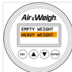
1. The screen pauses for three seconds with the display, “ENTER HEAVY – VEHICLE MUST BE HEAVY” before proceeding automatically to the next menu.
