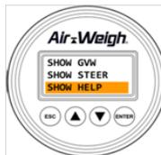
**Note:** You can turn off the How-To-Weigh instructions temporarily, until the next time you turn the truck off and on, by pushing either of the up/down arrows <▲▼> when the instructions are visible.
