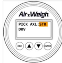
1. Using the up/down arrows <▲▼>, scroll to the proper empty weight identified from a certified scale ticket, then depress <ENTER>. The screen will briefly show Accepted to indicate its acceptance of the Heavy Weight.
