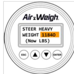
1. Press <ESC> to return to the PICK AXL menu and choose another axle for entering its Heavy Weight calibration.
